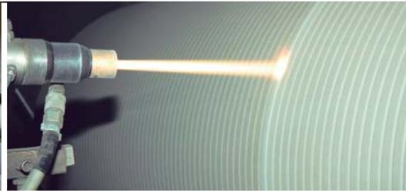
Spray coating on immersed roll
