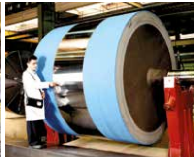
Conductor roll for electro galvanizing line
