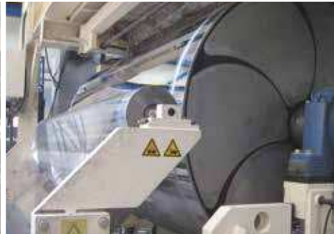
Chill roll for BOPP packaging film
