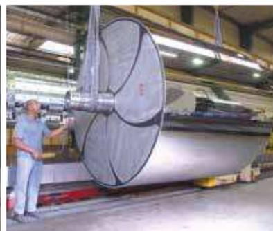
电容膜线及BOPET光学膜线等激冷辊
