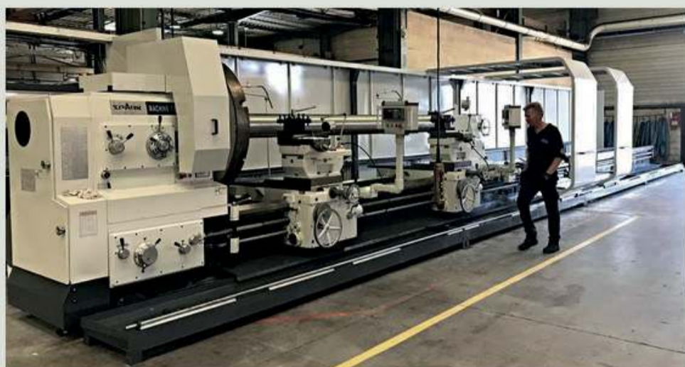
PMG POLIMIROIR : new lathe of 15 m.
