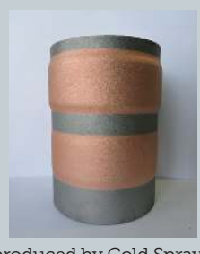
Dense deposit (porosity <0.2%) of copper produced by Cold Spray at OUEST COATING
