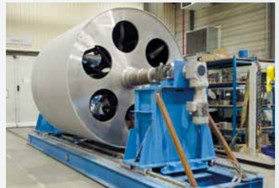
Chill Roll of Ø 2 300 mm with rough hard coat
