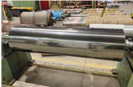
Calender Roll with hard coat poliglossy finish
